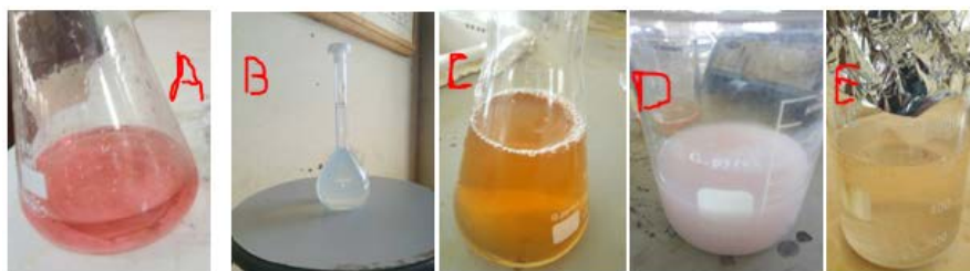
Figure 1. 0.01 M \text{CoCl}_2 (A), 0.01 M \text{Ag}(\text{NO}_3) (B), Aqueous root extract Palmyra palm (C), Mixture of Ag-Co immediately after addition (D), and Ag-Co BMNPs formation (E).
