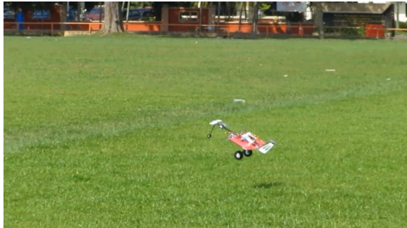
Figure 11. The ATRS-45 performing a near vertical landing using the retarded harrier maneuver.
