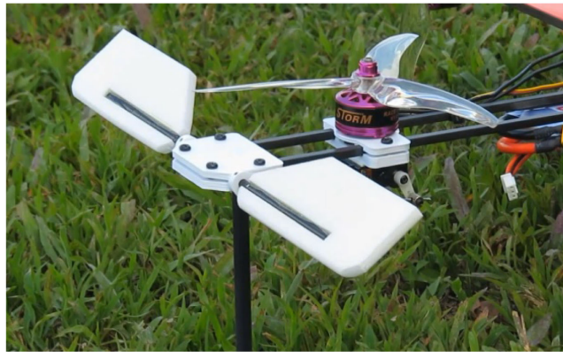
Figure 8. Addition of canard surfaces for pitch control during forward flight.
